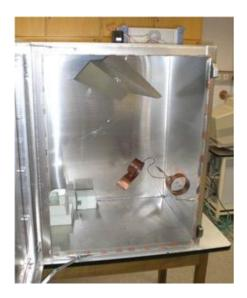
Fig.1: Small size ERC used for testing.
