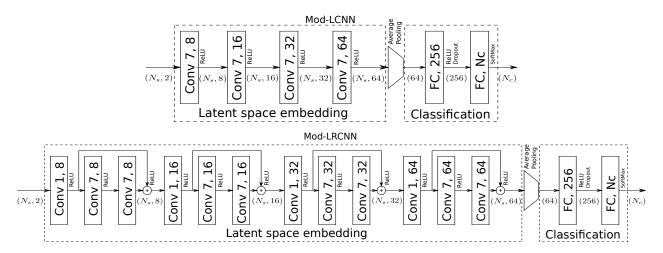
Figure 1 – Architecture of Mod-LCNN (top) and Mod-LRCNN (bottom), the neural networks developed in this study.  $N_s$  is the number of samples: 128 or 1024 in this study,  $N_c$  is the number of output classes: 7, 10, 11 or 24 in this study. The 1-dimensional convolutions have a kernel size of 7. During training the dropout rate is 0.5.
