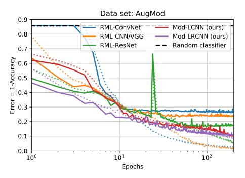
Figure 2 – Error rate as a function of the number of epochs for the five different neural network architectures, compared with the performances of a random classifier. Solid curves are for the test set and dotted curves for the training set. The comparison is performed with the AugMod data set on 1024 samples long signals.
