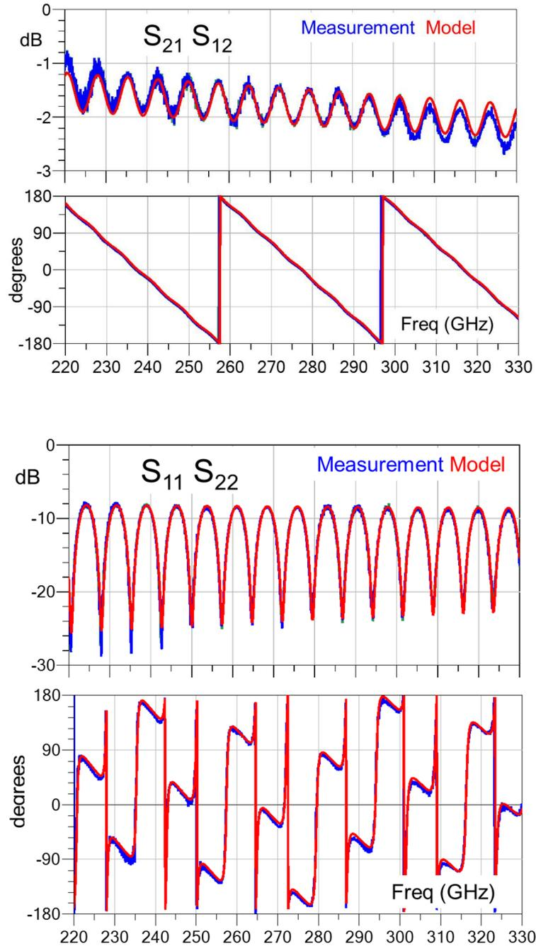
Fig 5 : Comparison between measured and simulated S parameters of the Rexolite slab in the J band
