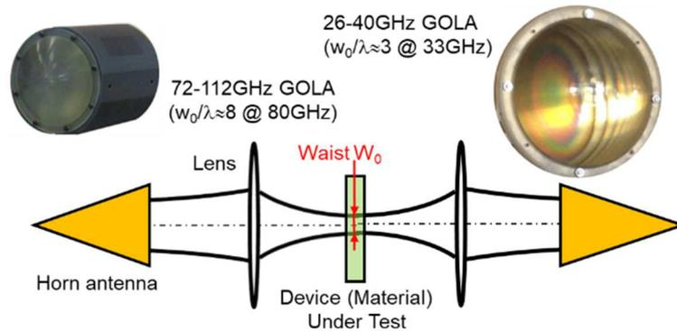
Fig. 2 : Gaussian beam focused to obtain the waist
