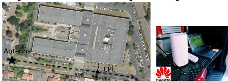
**Figure 1 :** on the left, satellite view of the 5G site at Bordeaux-Mérignac, position of the CPE receiving the data and axis of measurements; and on the right, CPE custom premise equipment used to receive the 5G data.
