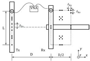
Figure 1: Schematic overview of the measurement setup.
