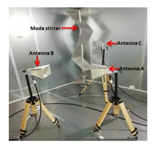
Figure 1 – Experimental setup in ESYCOM laboratory RC.
