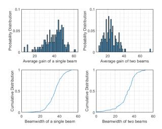
Figure 2. Gain and HPBW distributions for one and two-beam cases
