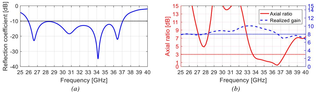
Figure 2 : Results : (a) Simulated reflection coefficient of the CP UWB antenna, (b) Realized gain and axial ratio of the CP UWB antenna
