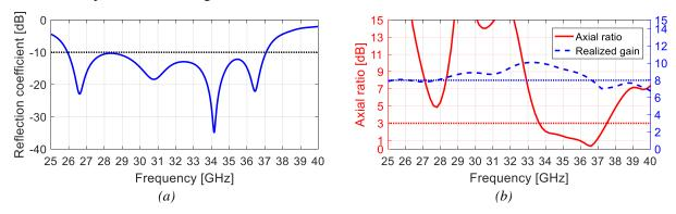
Figure 2 : Results : (a) Simulated reflection coefficient of the CP UWB antenna, (b) Realized gain and axial ratio of the CP UWB antenna
