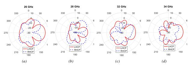
Figure 3 : Radiation pattern of the CP antenna in the YoZ-plane at: (a) 26 GHz, (b) 28 GHz, (c) 32 GHz and (d) 34 GHz
